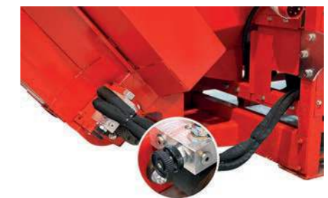
Outfeed conveyor speed control valve as easy-to-install accessory comes as standard equipment.
