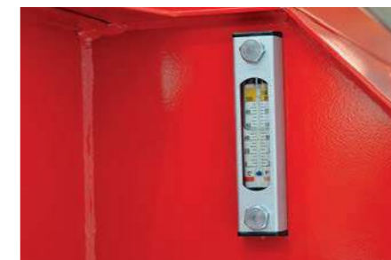
Large oil tank capacity and sight glass.
