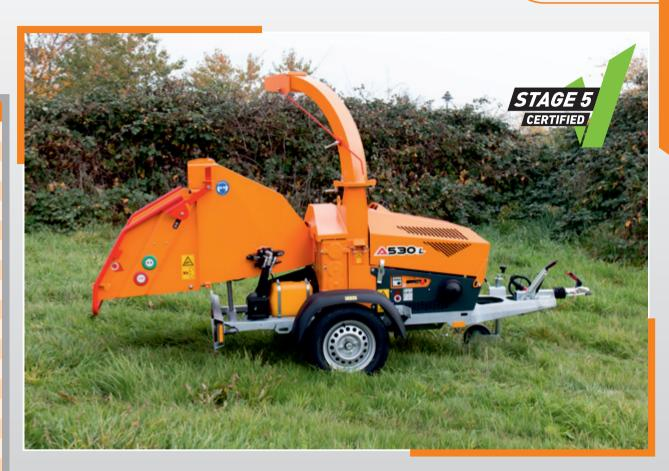
Available with braked or unbraked chassis. The 530L Di is a very popular and robust machine, weighing sub 750kg.
