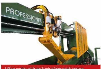
Lifting pusher with mechanical/pneumatic system
