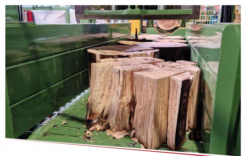
The automatic vertical splitting station (TB 600) is capable of processing logs of any diameter between 300 and 600 mm.
