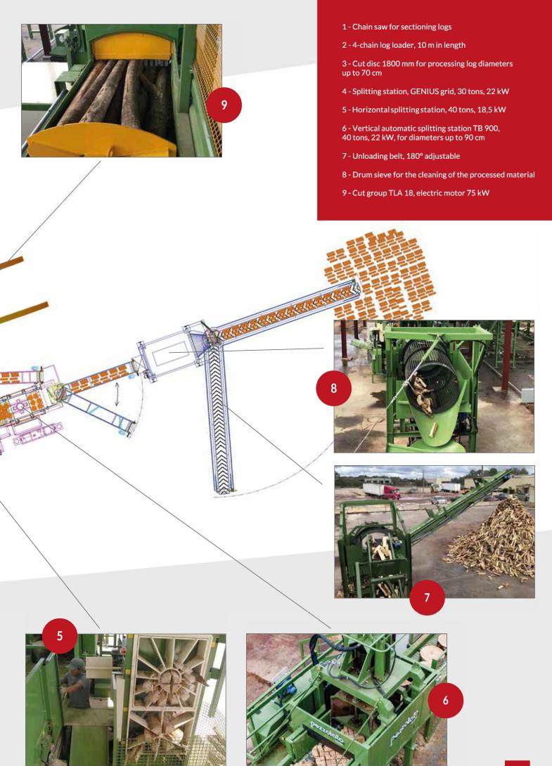
Industrial machinery with integrated log splitter, designed to produce firewood with the use of a variable number of operators from one to three, depending on the configuration.
