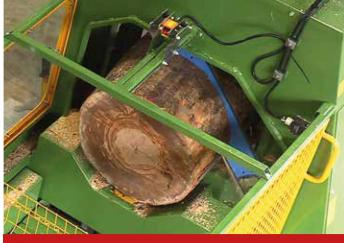
Photocell for automatic log length measurement
