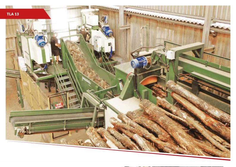
After cutting, the logs fall in a cumulating S-shaped conveyor (with closed meshes), which transfers them in front of the wood splitter.
